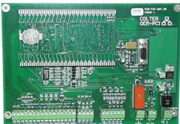
Rear view of the press batch controller showing the specially designed I/O board in more detail, also shown in the top left quarter of the board is the FMT-100 CPU board
