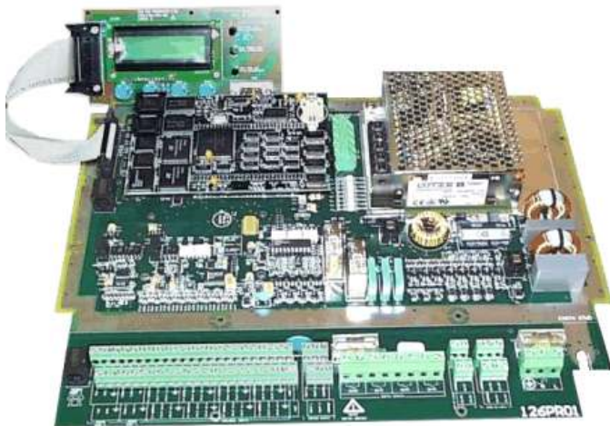
A view of the boiler control unit design. The standard CPU card can be seen in the top left of the large board. The LCD display and push buttons can be seen in the far top left.
